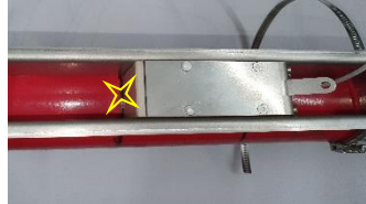
Figure 11: Attaching the transducer to marker 1
