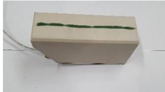
Figure 10: Application of the coupling gel
