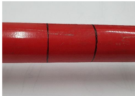
Figure 4: Marking the mounting position of the second transducer using a template
