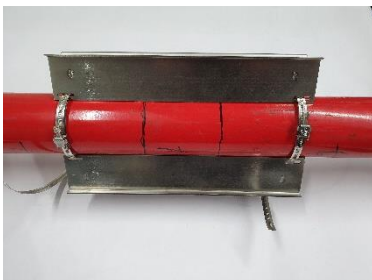
Figure 8: Fixation of the rails with metal tape
